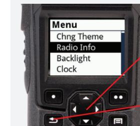
4. Press the **Up/Down Buttons** to highlight the desired mode. Then press the menu button to select that mode.
