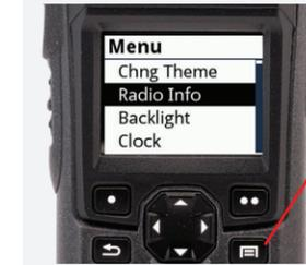
1. Press The **Menu Button** to select the Menu mode. The selectable menu parameters are then displayed below the menu as shown.
