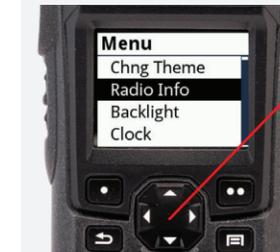
2. Press The **Up/Down Arrow** to scroll up or down through the list until the parameter you want to change is highlighted by the bar.
